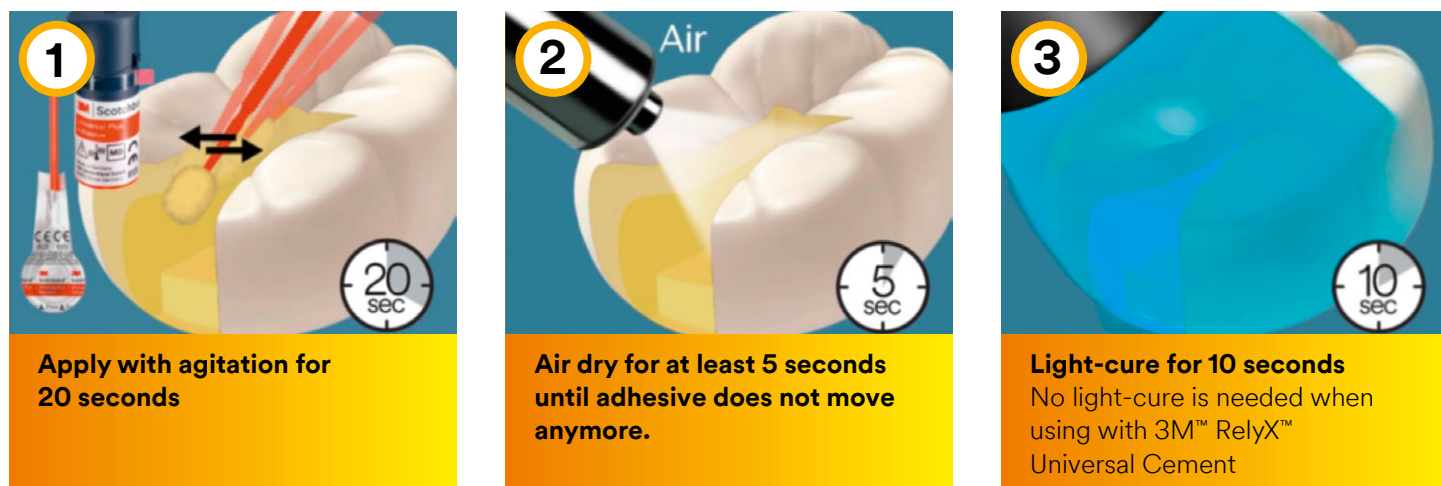
Fig. 34: Schematic illustration of application of 3M™ Scotchbond™ Universal Plus Adhesive
