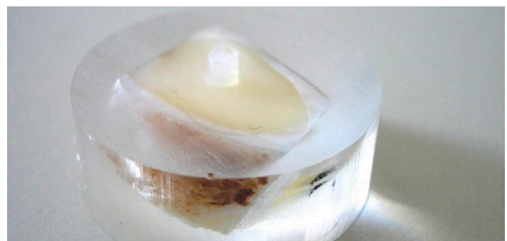
Fig. 4: Specimen for shear bond strength testing according to ISO 29022:2013 (bovine dentin)
