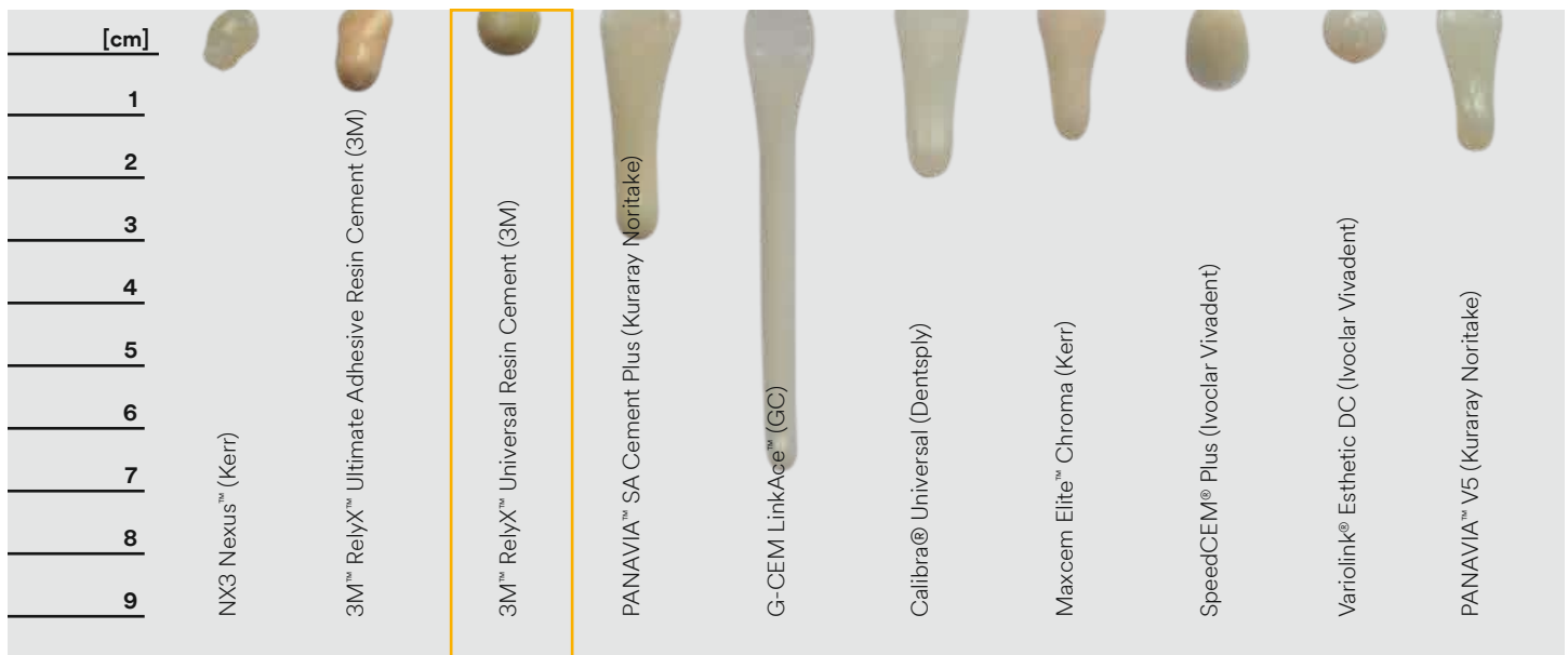
Fig. 2: To compare the flow properties, equal amounts of each cement were applied on a pad which was stored upright at 36°C/96.8°C for 2 minutes before the cement was light-cured.
