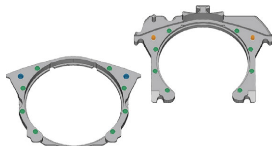
FIG. 33 CLEANING THE BLANK FRAME; MAGNETS MARKED GREEN, POSITIONING PINS MARKED ORANGE, RECESSES MARKED BLUE
