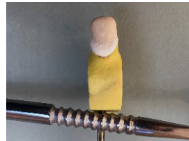
4. Vibrate to minimize the shrinkage
